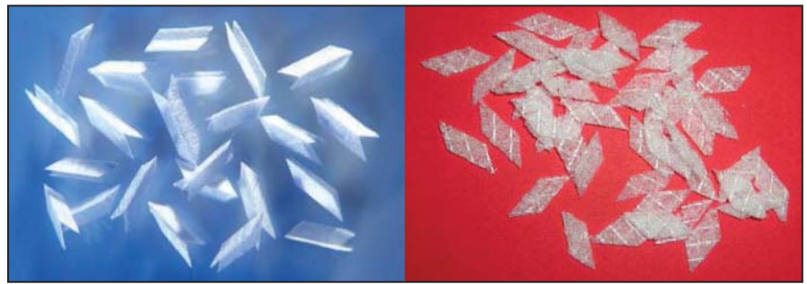
FIGURE 2. Bionoc II and Bionoc D carriers. Bionoc II (left): Made of 100% polyethylene terephthalate nonwoven fabric with treated surface; has high equivalent surface area (2,000 cm 2 /g carrier); is rigid and inert; and requires enzymatic treatment for cell removal. Bionoc D (right): Made of alginate base and soluble without requirement of enzymatic treatment for cell removal; has high equivalent surface area (1,500 cm 2 /g carrier); and requires serum in the medium.
