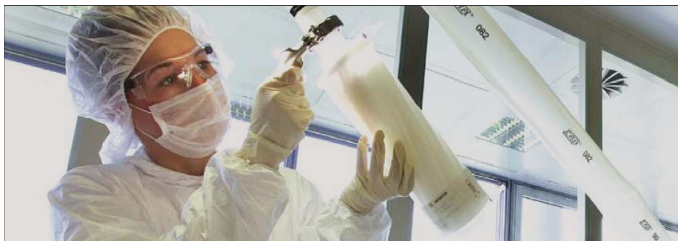
Figure 1. Disposable, single-use Sartobind® Q membrane chromatography setup.
