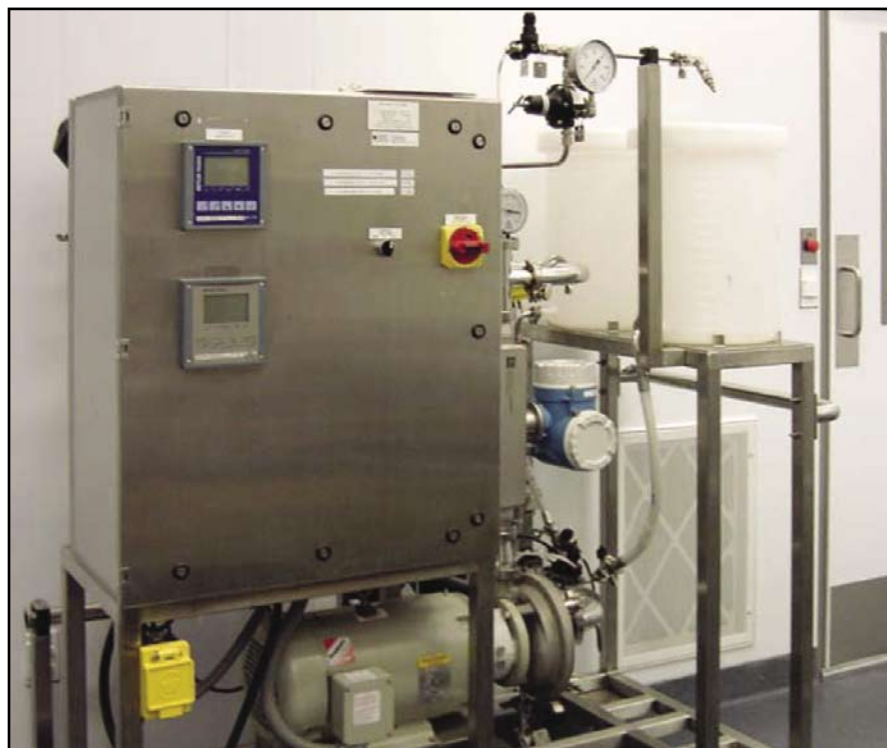
Figure 6. Mobile Clean-In-Place (CIP) cart: The dimension of the cart was carefully sized for easily maneuvering the unit within the suites.
