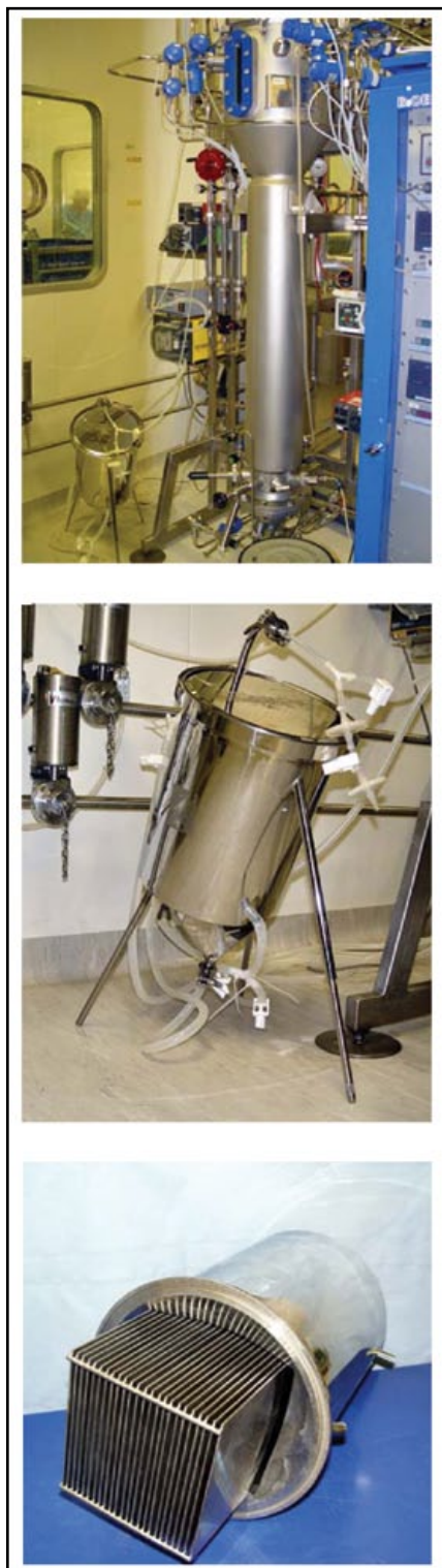
Figure 2. 50L airlift system and associated settler.
