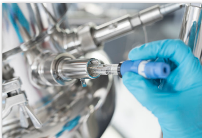
FIGURE 4. The Endress+Hauser CPS171D pH sensor has a glass membrane and reference gel that withstands SIP and CIP procedures.
