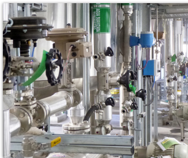
FIGURE 3. Calibrating sensors in a biomanufacturing plant often requires removal of the instrument for calibration in a laboratory setting.
