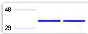
FIGURE 3. Caliper LC90 quantitation and virtual SDS-PAGE representation of the validation expression experiment. The DOE-predicted condition produced a 40% greater yield than the best condition from the model, and a 100% improvement to the RSD optimal yield over the small-scale experiment.
